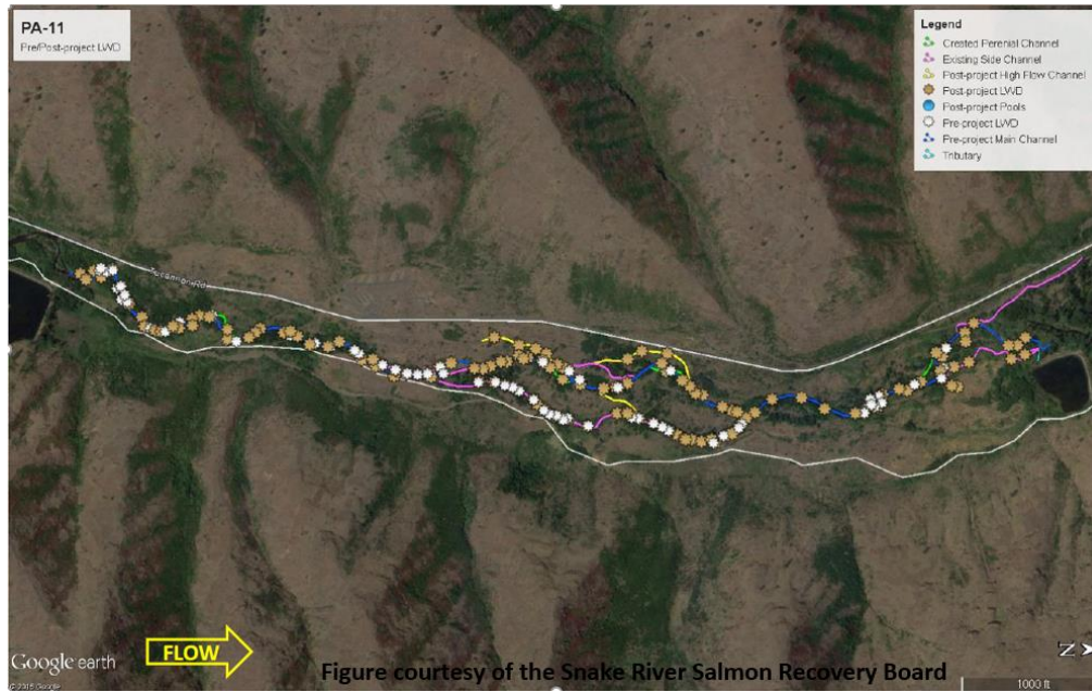
Figure 6. Project Area 11 pre and post-treatment conditions (from Rapid Habitat Surveys) for key LWD pieces and side channels. CHaMP post-treatment sample not available for this report.
