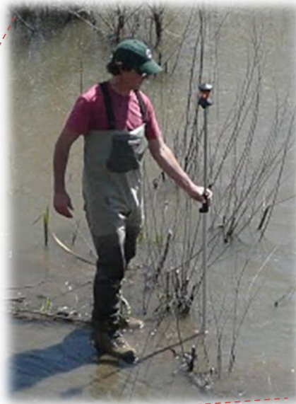
Crew member (rodman) with Survey Rod and prism
