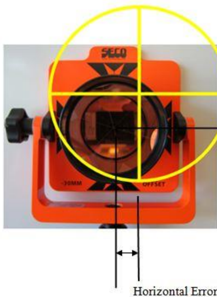
Incorrectly aimed Total Station
