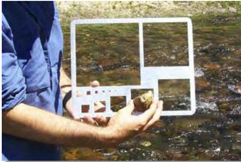
Figure 23. Gravelometer used to classify the b-axis of particles.
